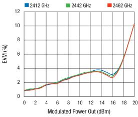
EVM vs. Modulated Power Out Across Frequency 802.11g, 54 Mbps, 64 QAM
