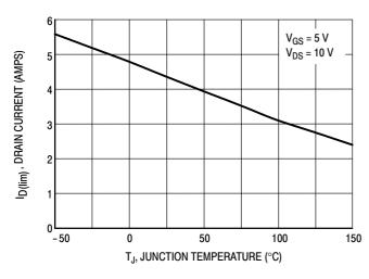
Figure 3. I<sub>D(lim)</sub> Variation With Temperature
