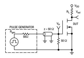
Figure 10. Switching Test Circuit
