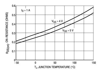
Figure 5. On-Resistance Variation With Temperature
