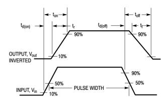
Figure 11. Switching Waveforms
