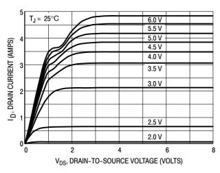
Figure 1. Output Characteristics
